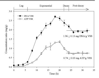
235.7  $\pm$  5.3 mg COD/l corresponding to 97.5% removal efficiency (Fig. 1). This could be because net microbial growth, and net synthesis of genetic and energy compounds for proliferation cease after the end of exponential growth (Shuler and Kargi 2002). Therefore, it would be possible to use the constant ratios as conversion factors to convert measured ATP and DNA concentrations into microbial mass in similar situations.
